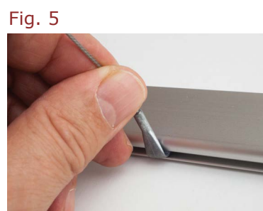
Fig. 5 Slip the end of the hanger into the track by raising it to a horizontal position. Rotate it down to a vertical position.
