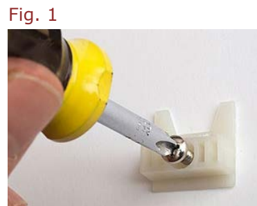
Fig. 1 Measure and mark carefully to ensure good alignment and level mounting, and tighten the mounting screw or bolt snugly.
