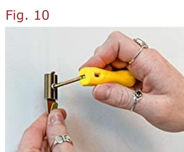
Fig. 10 Secure the hook in the desired position by tightening the hex screw with the included wrench.
