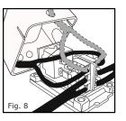
Measure from the junction box to the far end of the wall-mounted track, add a couple of inches to allow for connections, and cut a section of flat track cable to that length. Lav the cable temporarily in the wall track (without removing the tape's protective covering) and carefully strip away 1/2 inch (1 cm) of insulation at the junction box end.
