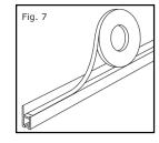
Using a rag or paper towel moistened with rubbing (isopropyl) alcohol, wipe clean the inner horizontal surface of the wallmounted track and allow to dry. If the track cable has attracted dust or grease, wipe it as well, and let dry.
