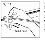
Continue holding wand base firmly against front of track and turn the wand lever clockwise to the horizontal position. Do not press the wand base down — let the lever do the work, drawing the wand's contact probes into the track cable. The lamp should then turn on. Repeat process for all wands.
