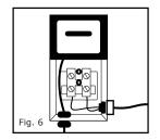
Now connect the other end of the cable to the power supply. Strip 1/2 inch (1 cm) of insulation from both conductors, feed through the cable holder, and insert the stripped ends into the two OUTSIDE terminal block screws. After securing, feed a few inches of cable into the case to provide for future repairs. Tighten cable holder and replace power supply cover. **Do not plug in to** AC power at this stage.
