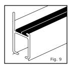
Working outward from the junction box, lift the cable slightly and start peeling away the protective strip to expose the adhesive. Work your way along the track, positioning the cable atop the tape as you go, ensuring that it lies flat. When fully in place, press the cable gently onto the tape to make sure it sits securely, and trim any excess at the end. If installing lights on both sides of the junction box, repeat for the other portion of track. Replace the cover on the junction box.
