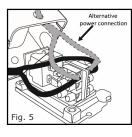
Route the cable as shown in Figure 5. Note the different paths depending on which end of the box the cable enters through; follow them carefully to ensure that the box cover reattaches properly.
